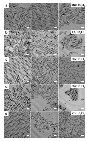
Fig. 8 TEM images taken of doped In<sub>2</sub>O<sub>3</sub> nanocrystals at varying molar dopant ratios. Scale bars are 20 nm. The nominal dopant percent in the precursor increases from left to right, 5% dopant on the left, 10% center, and 20% right: (a)  $Mn:In_2O_3$ , (b)  $Fe:In_2O_3$ , (c)  $Co:In_2O_3$ , (d)  $Cu:In_2O_3$ , and (e) Zn:ln<sub>2</sub>O<sub>3</sub>. Reproduced from ref. 45 with permission from ACS, copyright 2017.
