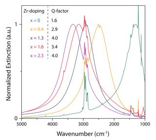
Fig. 14 Optical extinction spectra of different  $Zr:In_2O_3$  NCs displaying narrow and symmetric LSPR bands increasing in energy with an increase in Zr doping. Spectra were taken by FTIR of NCs dispersed in tetrachloroethylene. Reproduced from ref. 52 with permission from ACS, copyright 2019.
