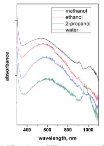
Fig. 22 UV-vis-NIR absorbance of  $WO_{3-x}$  nanocrystals – LSPRs in different protic polar solvents. Reproduced from ref. 70 with permission from RSC, copyright 2016.
