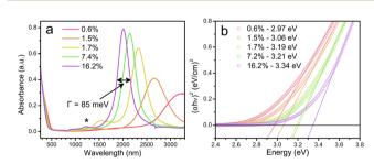
Fig. 24 (a) Solution-phase spectra of ICO nanocrystals dispersed in CCl<sub>4</sub> for five levels of % atomic doping of In. The fwhm or  $\Gamma$  is indicated for the 16.2% doped sample. (b) Plots of  $(\alpha h \nu)^2$  vs. photon energy (eV) for five samples of spherical ICO nanocrystals. Open circles are measured data, dotted lines are linear fits, and the legend shows the extracted direct bandgap energies. Reproduced from ref. 71 with permission from ACS, copyright 2013.
