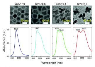
Fig. 9 Solution-phase UV-vis-IR absorbance spectra of four shapes (spheres, triangles, tripods and tetrapods) of Sn-doped nanocrystals in CCl<sub>4</sub>. The nominal doping concentration is the same (8%) for all the samples and the real doping concentrations are 7.9%, 8.6%, 8.4%, and 8.3%, respectively, determined by ICP-AES techniques. Reproduced from ref. 53 with permission from RSC, copyright 2017.
