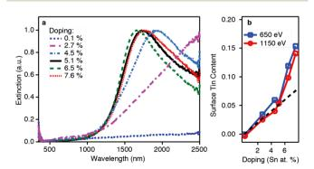
Fig. 11 (a) Optical extinction and (b) XPS depth profiling versus doping for the doping series. The dotted black line in panel (b) shows the expected Sn/(In + Sn) ratio for a uniform doping profile. Reproduced from ref. 51 with permission from ACS, copyright 2014.
