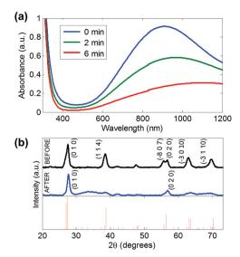
Fig. 20 (a) UV-vis-NIR absorption spectra of WO<sub>2.83</sub> nanorods in Nmethylpyrrolidone upon heating at 175 °C in air for 0, 2, and 6 min. (b) XRD patterns of  $WO_{2.83}$  nanorods in N-methylpyrrolidone (top) before and (middle) after heating at 175 °C for 6 min in air and (bottom) the reference pattern for WO<sub>2.83</sub>. Reproduced from ref. 15 with permission from ACS, copyright 2012.
