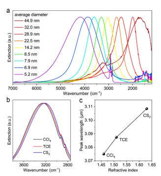
Fig. 25 (a) Normalized extinction spectra of size controlled CdO NCs synthesized with different HMDS/Cd ratios. (b) Extinction spectra of CdO NCs (8.5  $\pm$  1.2 nm) dispersed in different solvents. (c) Plot of LSPR peak wavelength *versus* the refractive index of solvent. CCl<sub>4</sub>: carbon tetrachloride, TCE: tetrachloroethylene, CS<sub>2</sub>: carbon disulfide. Reproduced from ref. 73 with permission from ACS, copyright 2020.
