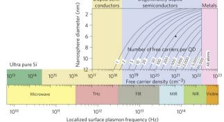
Fig. 1 Localized surface plasmon resonance (LSPR) frequency dependence on free carrier density and doping constraints. Reproduced from ref. 11 with permission from Springer Nature, copyright 2011.
