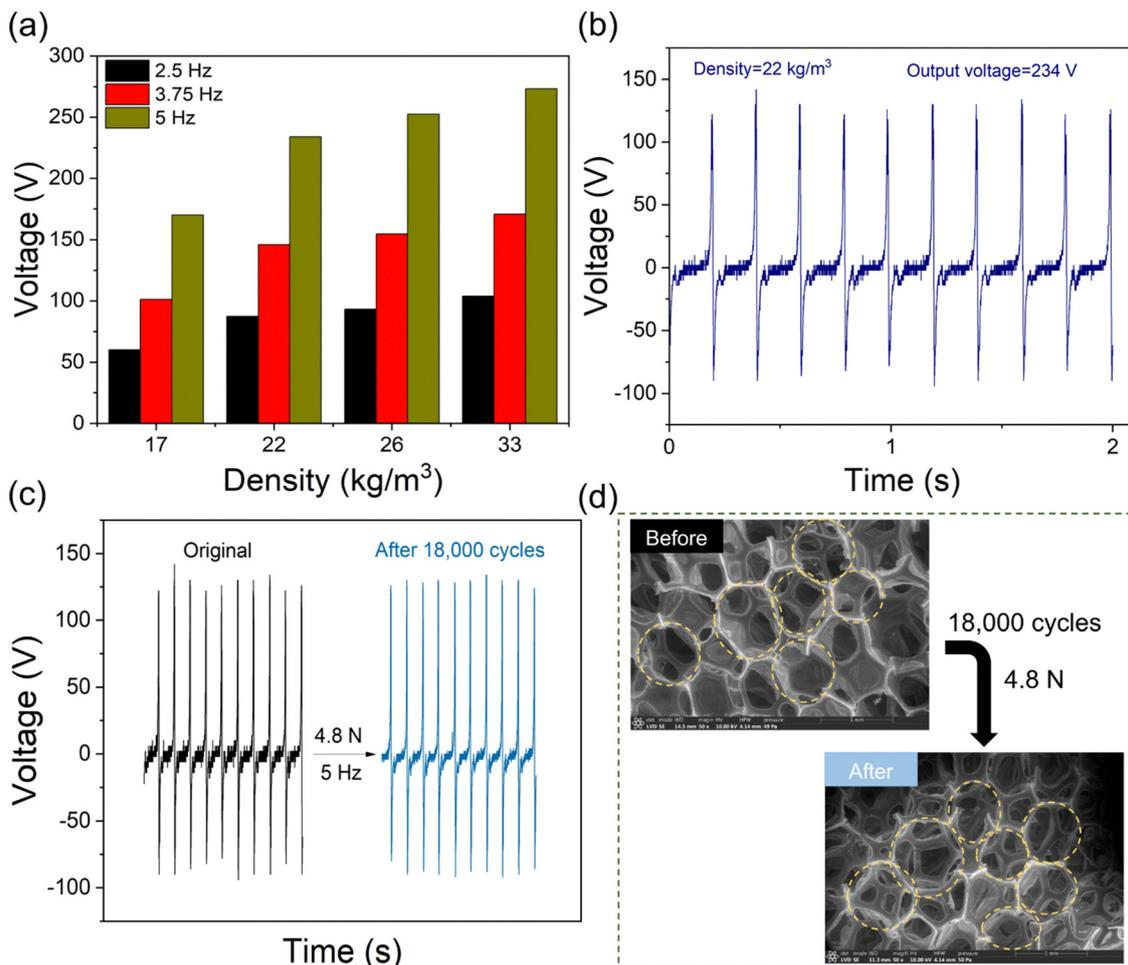
Fig. 7 (a) Density of FPU versus output voltage of TENG at a thickness of 4 mm; (b) output voltage of FPU foam with a density of 22 kg m<sup>-3</sup> and a thickness of 4 mm under a force of 4.8 N and frequency of 5 Hz; (c) durability test of FPU.15-based TENG over 18 000 contact-separation cycles at an applied force of 4.8 N; and (d) SEM analysis of FPU foam before and after 18 000 cycles.
