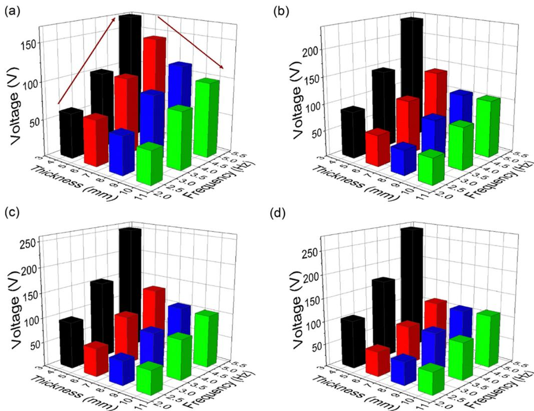
Fig. 8 The relationship between the thickness of the FPU, applied frequency and output voltage of TENG for four different densities: (a) 17, (b) 22, (c) 26, and (d) 33 kg m<sup>-3</sup>.
