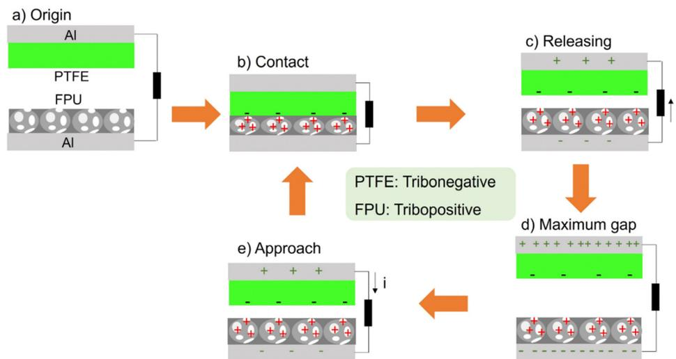
Fig. 6 (a)–(e) Schematic illustration of the operating principle of the FPU-based TENG in vertical contact-separation mode.
