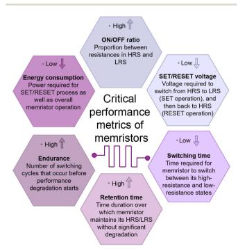
Fig. 4 Critical parameters for evaluation of the performance of
