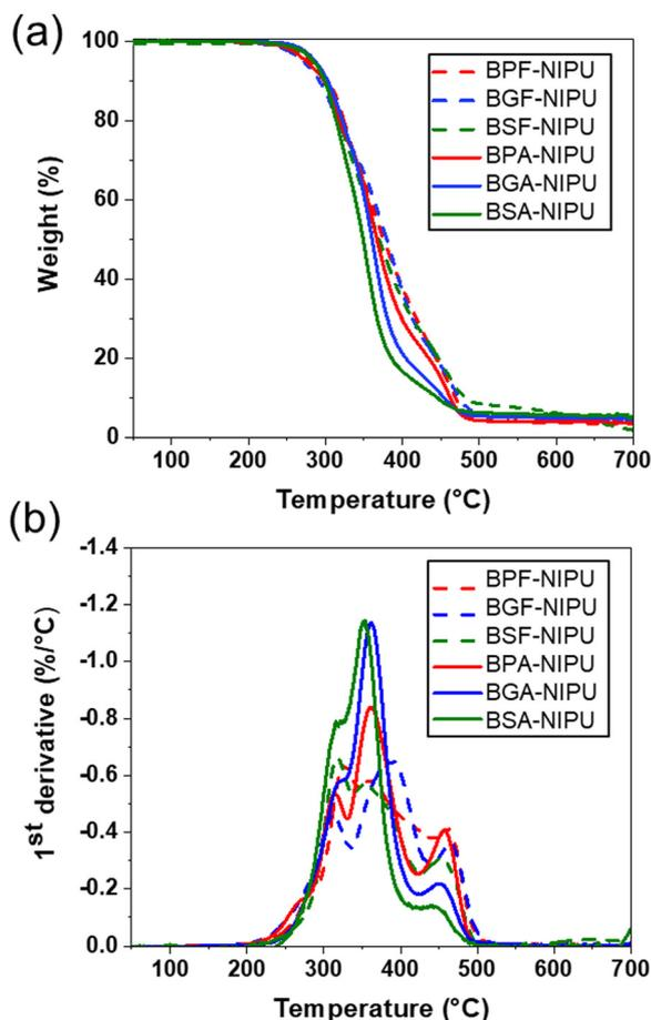
Fig. 4 (a) TGA thermograms of NIPUs in  $N_2$  atmosphere; sample weight (%) as a function of temperature with a heating rate of  $10$  °C  $min^{-1}$ , and (b) the first derivative of the weight remaining (%/°C) as a function of temperature for all NIPUs.
