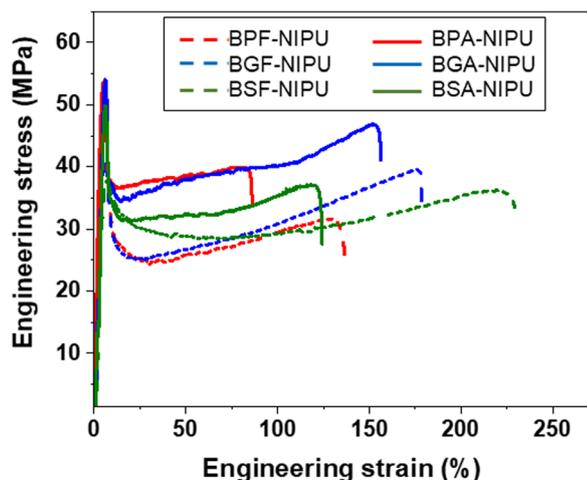
Fig. 2 Representative tensile engineering stress vs. engineering strain curves for NIPUs acquired from uniaxial tensile testing using a load cell of 100 N and a strain rate of 10% min<sup>-1</sup> at ~20 °C.
