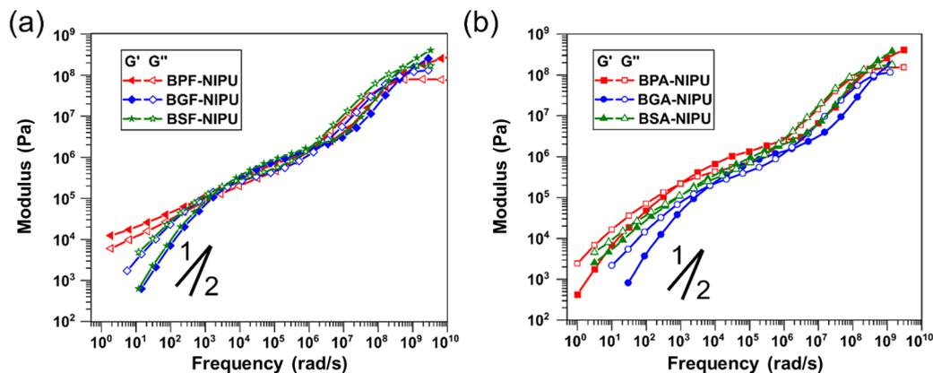
Fig. 5 Frequency-dependent storage ( $G'$ ) and loss ( $G''$ ) moduli for (a) unsubstituted bridging carbon- and (b) dimethyl-substituted bridging carbon-based NIPUs. The master curves were constructed using time-temperature superposition and reported at 150 °C. Lines indicate typical power-law scalings of  $G'$  (slope of 2) and  $G''$  (slope of 1).
