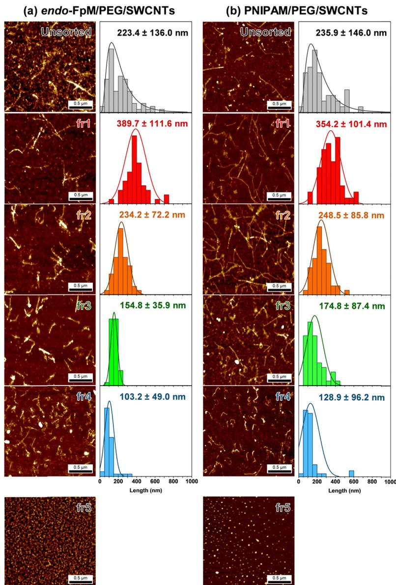
Fig. 3 AFM images and length distribution of unsorted, fr1, fr2, fr3, fr4, and fr5 of (a) *endo*-FpM/PEG/SWCNTs and (b) PNIPAM/PEG/SWCNTs. Displayed values are mean length  $\pm$  standard deviation for  $N = 50$ .
