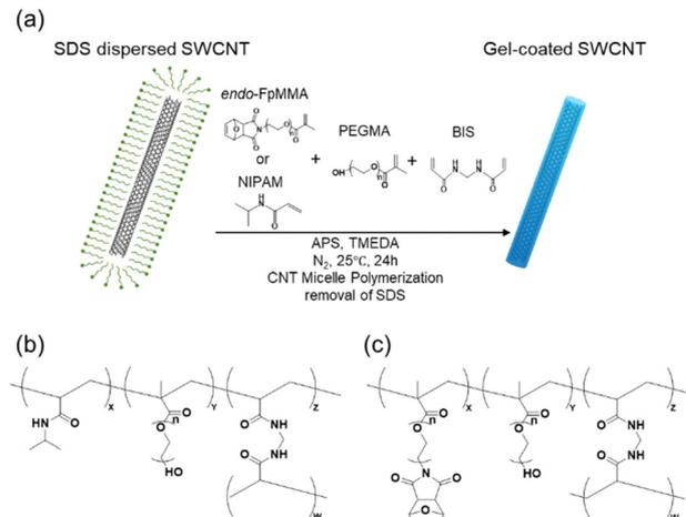
Fig. 1 (a) Scheme of the synthesis of gel-coated SWCNTs by CNT micelle polymerization. Chemical structure of the cross-linked polymer in (b) PNIPAM/PEG/SWCNTs and (c) *endo*-FpM/PEG/SWCNTs.
