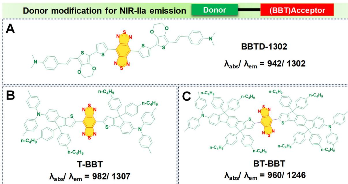
**Fig. 5** Donor modification for NIR-IIa emission using the BBT acceptor core with molecular structures of (A) BBTD-1302; (B) T-BBT; and (C) BT-BBT fluorophores with their absorption and emission values.
