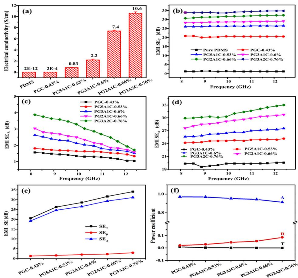
**Fig. 10** (a) Electrical conductivity and (b)  $SE_T$  of PDMS, PGC-0.43% and PGACs in the X-band; (c)  $SE_R$ , (d)  $SE_A$ , (e) the average  $SE_T$ ,  $SE_R$ ,  $SE_A$ , and (f) the average power coefficients (A, R, T) of PGC-0.43% and PGACs in the X-band; reproduced with permission from ref. 94, copyright reserved Elsevier 2019.
