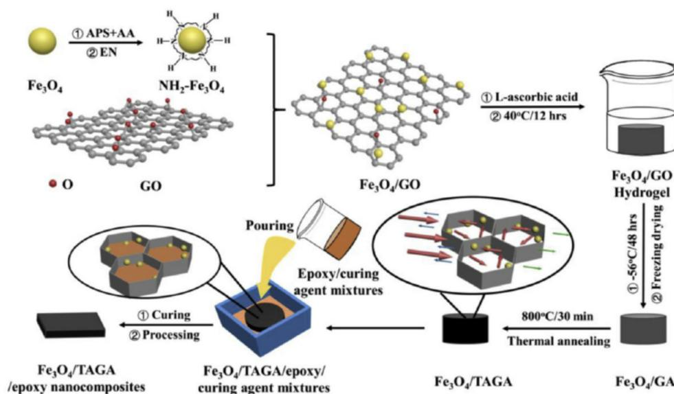
Fig. 11 The schematic for the fabrication of the Fe<sub>3</sub>O<sub>4</sub>/TAGA/epoxy nanocomposites; reproduced with permission from ref. 104, copyright reserved Elsevier 2019.
