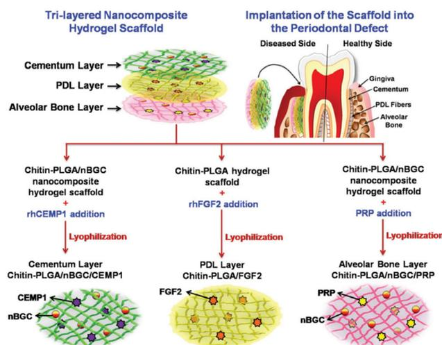
**Fig. 3** Schematic description of the development of a three-layer nanocomposite hydrogel scaffold and its implantation into a periodontal defect for concurrent and complete periodontal regeneration. Reproduced from ref. 184 with permission from Wiley-VCH GmbH, copyright 2017.
