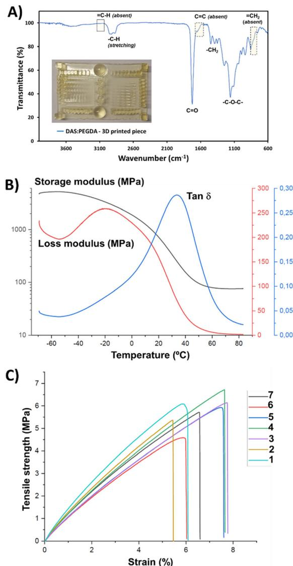
**Fig. 7** (A) FTIR-ATR spectrum of the 3D-printed piece shown in the inset image. (B) DMA analysis of the DAS : PEGDA copolymer. (C) Stress-strain curves of DAS : PEGDA copolymer dumbbell samples. Both assays were performed with samples DLP printed under UV light and after post-curing processes.
