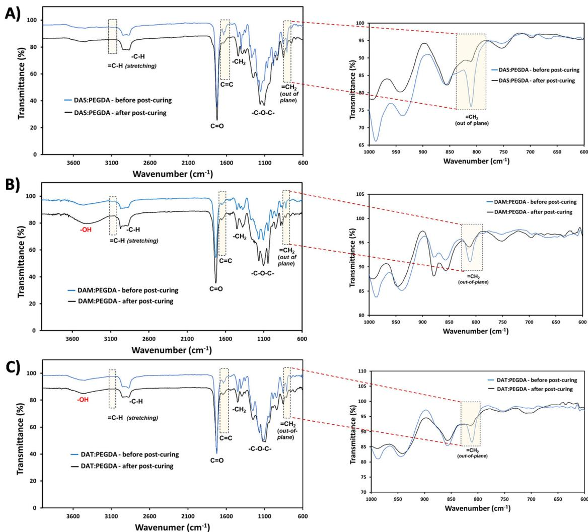
**Fig. 4** FTIR-ATR spectra comparing the samples before and after the post-curing process: (A) DAS : PEGDA; (B) DAM : PEGDA; and (C) DAT : PEGDA copolymers. On the right, the detail of the  $=\text{CH}_2$  out-of-plane bending bands, which overlapped evidencing that the polymerization reaction was complete.
