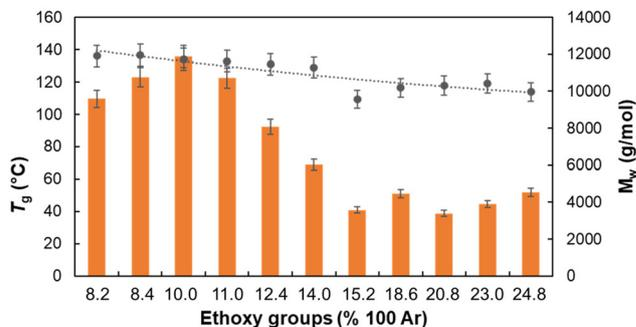
Fig. 4 The correlation between EtO-groups content, *M<sub>w</sub>* and resulting *T<sub>g</sub>* values. ●- *T<sub>g</sub>* values ■- *M<sub>w</sub>*.
