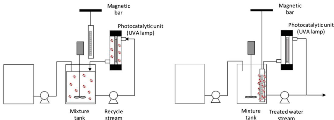
**Fig. 8** (a) Challenges of MRNPCs in practical applications; (b) operation of magnetic photocatalytic reactor: 1) loading of MRNPCs and water, 2) continuous phototreatment; 3) end of phototreatment, 4) MRNPCs recycling. Reproduced from ref. 70 with permission from Elsevier, copyright 2019.
