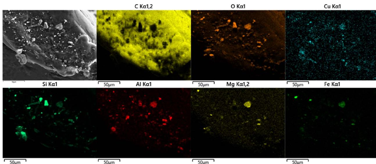
Fig. 6 SEM images of PS-lake and its corresponding EDX mappings for C, O, Cu, Si, Al, Mg and Fe.
