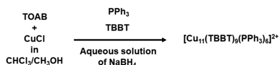
Fig. 6 Synthesis procedure of [\text{Cu}_{11}(\text{TBBT})_9(\text{PPh}_3)_6]^{2+} NC.
