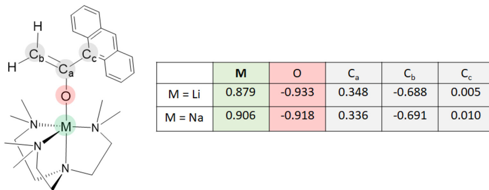
Fig. 6 NBO charge per atom from natural population analyses of 6' -Li and 6' -Na.
