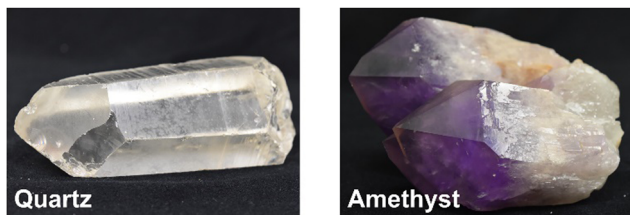
Fig. 1 Colour variation in quartz caused by isomorphous substitution; amethyst is quartz containing a trace amount of iron. Permission for photography was given by Mineral Industry Museum of Akita University. The archive number is 292 and 14277 for quartz and amethyst, respectively.
