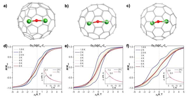
Fig. 6 Molecular structures of  $Dy_2O@C_s(6)-C_{82}$  (a),  $Dy_2O@C_3(8)-C_{82}$  (b) and  $Dy_2O@C_{2v}(9)-C_{82}$  (c). Magnetic hysteresis curves of  $Dy_2O@C_s(6)-C_{82}$  (d),  $Dy_2O@C_{3v}(8)-C_{82}$  (e) and  $Dy_2O@C_{2v}(9)-C_{82}$  (f) in the range of 1.8-7 K using a field sweep rate of 2.9 mT s<sup>-1</sup>. The insets represent their corresponding ZFC/FC curves at an applied magnetic field of 0.2 T with a temperature sweep rate of 5 K min<sup>-1</sup>. Reproduced from ref. 102.
