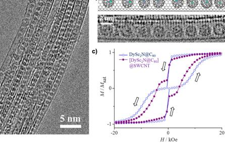
Fig. 11 (a) and (b) TEM images and structural model of [DySc<sub>2</sub>N@C<sub>80</sub>]@SWCNT. (c) Magnetic hysteresis loops for DySc<sub>2</sub>N@C<sub>80</sub> (open circles) and [DySc<sub>2</sub>N@C<sub>80</sub>]@SWCNT (filled circles) at 1.8 K. Arrows indicate the direction of the measurements. Reproduced with permission from ref. 236 (Copy right 2018, American Chemical Society).
