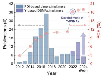
Progress in photovoltaic performances of PSCs based on PDI- and Y-based oligomer acceptors during the past years.
