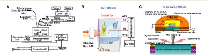
Fig. 8 Schematics of the combined base of simultaneous STM and Raman spectroscopy (A), in situ cell of EC-TERS (B) and nano-FTIR (C), respectively. (A) is reproduced with permission from ref. 110. Copyright 1996 Elsevier. (B) is reproduced with permission from ref. 34. Copyright 2015 American Chemical Society. (C) is reproduced with permission from ref. 36. Copyright 2019 American Chemical Society.
