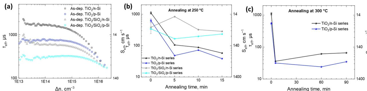
Fig. 2 (a) Injection-level dependent effective lifetimes for Si wafers passivated by 54 nm thin films of (a) as-deposited  $\text{TiO}_2$ , (b) annealed  $\text{TiO}_2$  films at 250 °C, and (c) annealed  $\text{TiO}_2$  films at 300 °C for different durations. The corresponding surface recombination velocities ( $S_{\text{eff}}$ ) are also shown on the right y-axis.
