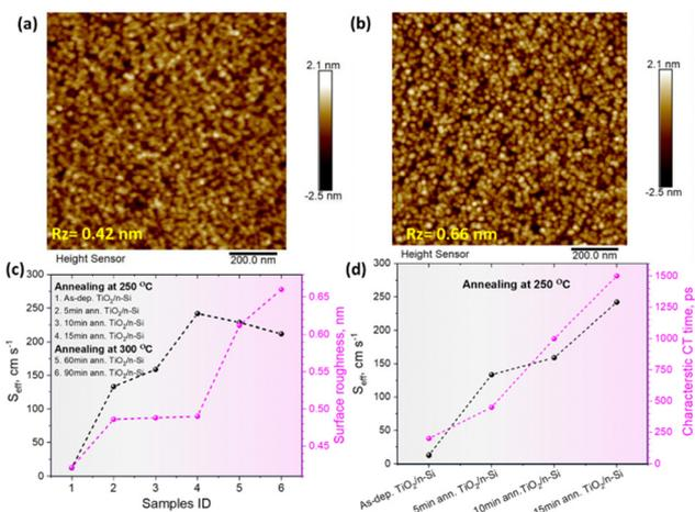
Fig. 7 AFM images of (a) as-dep.  $\text{TiO}_2/\text{n-Si}$ , (b) 90 min annealed  $\text{TiO}_2/\text{n-Si}$  at 300 °C, (c) correlation of surface recombination velocity and surface roughness of the samples, and (d) correlation of surface recombination velocity and characteristic charge transfer times for HF-treated  $\text{TiO}_2/\text{n-Si}$  heterojunctions annealed at 250 °C up to 15 minutes.
