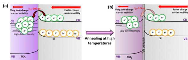
Fig. 6 Schematic of photoinduced interfacial charge transfer in (a) as-dep. TiO<sub>2</sub>/n-Si and (b) 15 min annealed TiO<sub>2</sub>/n-Si samples.
