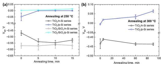
Fig. 3 Surface barrier height of different series of TiO<sub>2</sub>/Si heterojunctions deposited at 120 °C and further annealed at (a) 250 °C and (b) 300 °C for different time durations.
