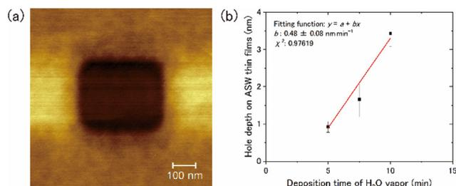
**Fig. 2** (a) AFM image of a square hole made by strong tunnelling current using a scanning tunnelling microscope. (b) The relationship between hole depth and deposition time at 15 K. The red line represents the result of data fitting using a linear function.
