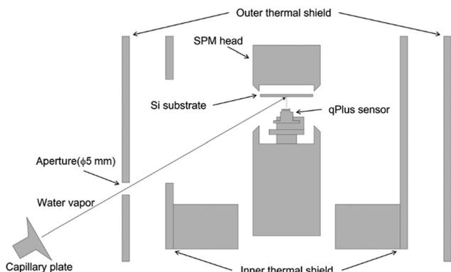
**Fig. 1** Schematic of the inside of the observation chamber. The SPM head is surrounded by the inner 10 K and the outer 100 K thermal shields. Water vapor at room temperature is deposited after passing through a 5 mm-diameter aperture on the outer shield with an incident angle of  $60^\circ$  to the substrate.
