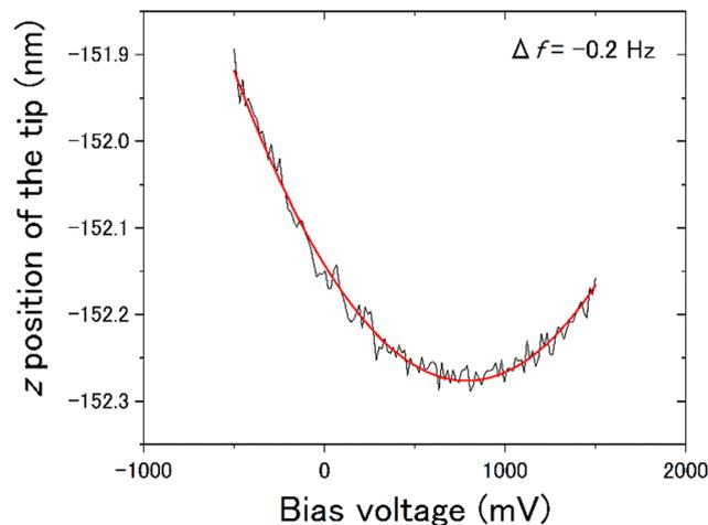
**Fig. 3**  $V_{\text{Bias}}$  dependence of  $z$ -positions of the tip at a single measurement point on ASW at 15 K while maintaining a constant frequency shift of  $\Delta f = -0.2 \text{ Hz}$ . Lower  $z$  values indicate that the tip positions are closer to the ASW surface. The fitting function (red curve) was a quadratic function. The bias voltage at the vertex of the quadratic function indicates a negative  $V_{\text{LCDP}}$  at the measurement point.
