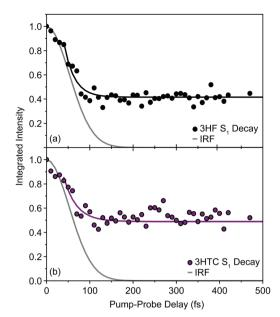
**Fig. 3** Spectral dynamics of (a) 3HF and (b) 3HTC for the S<sub>1</sub> OH bend transitions near 1275 cm<sup>-1</sup>. The data were fit to a monoexponential decay function,  $f(t) = Ae^{-t/\tau} + b$  (solid lines). The exponential decay time constants (24 ± 3 fs for 3HF and 29 ± 8 fs for 3HTC) are convolved with the instrument response (grey trace) and, therefore, are characterized as being sub-100 fs.
