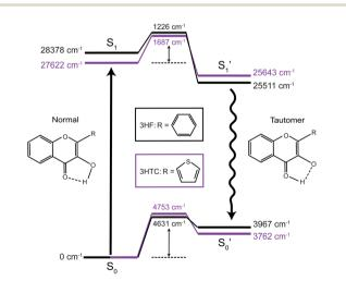
Fig. 1 Calculated energy level diagrams for 3HF (black) and 3HTC (purple). Barrier heights relative to the  $S_0$  and  $S_1$  normal states are shown for the transition state levels. Calculations were performed at the B3LYP-D3BJ/aug-cc-pVDZ level of theory and basis set.
