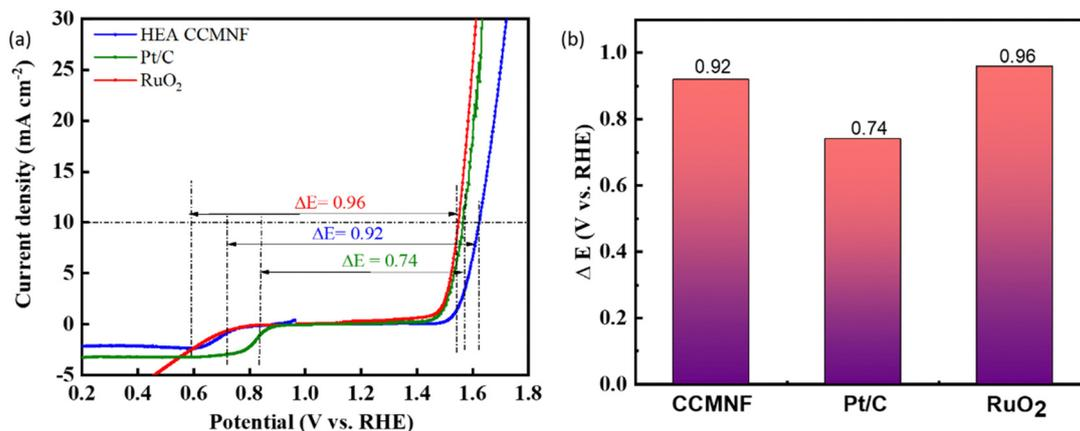
Fig. 5 (a) LSV plots depicting the calculation of  $\Delta E$  as the difference between the potential required to reach  $10 \text{ mA cm}^{-2}$  current density in the OER ( $E_{j=10}$ ) and the potential at the half-wave of the ORR curve ( $E_{1/2}$ ). (b) The obtained  $\Delta E$  values for different catalysts describing their bifunctional activity.
