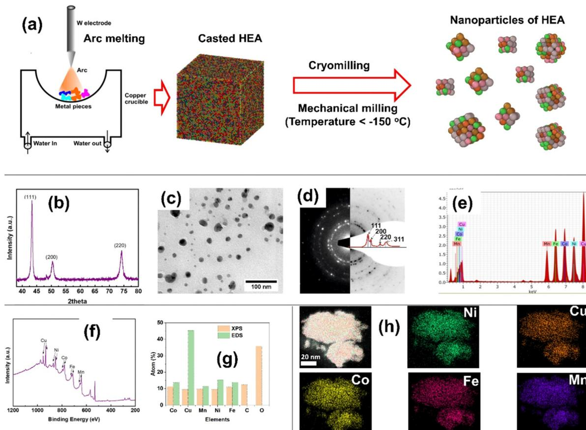
**Fig. 1** (a) Schematic of nanocrystalline HEA preparation by casting-cum-cryomilling, (b) X-ray diffraction peaks of the nanocrystalline CCMNF alloy, (c) bright-field TEM micrograph of CCMNF nanocrystalline powder, (d) ring diffraction pattern of a selected area of the nanoparticles, (e) EDS spectrum produced through TEM associated EDAX, (f) survey spectrum of CCMNF nanoparticles by XPS, (g) composition comparison between XPS and EDS, and (h) EDS elemental mapping by EDAX associated in TEM.
