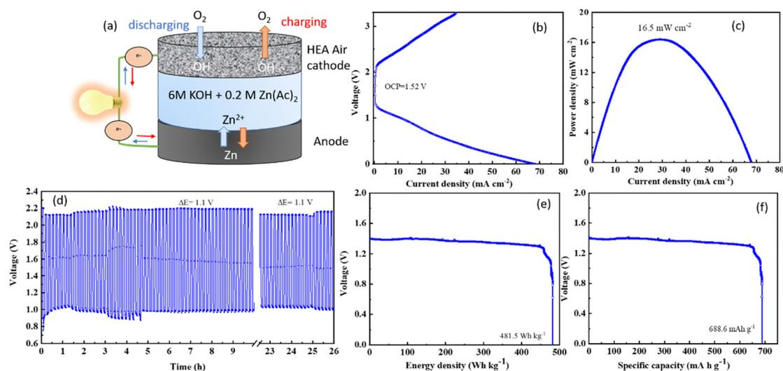
Fig. 6 (a) A schematic representing the aqueous zinc–air battery set-up, (b)  $i$ – $v$  polarization curve of CCMNF zinc–air battery depicting its open-circuit voltage. Various evaluation parameters to assess the performance of the zinc–air battery: (c) power density measurements, (d) galvanostatic charging and discharging at  $5 \text{ mA cm}^{-2}$  current density, (e) energy density, and (f) specific capacity measurements are presented.
