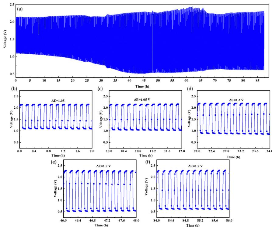
Fig. 7 (a) Long-term charge–discharge cycles of CCMNF supporting its excellent performance as an oxygen electrocatalyst in the zinc–air battery, (b)–(f) the changing  $\Delta E$  values over the continuous charging–discharging operation.
