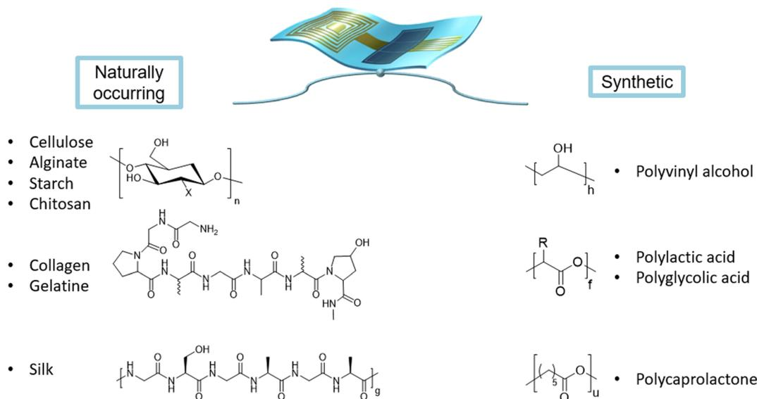
Fig. 4 Bioderived supporting materials for electronics-polysaccharides (cellulose,<sup>48,56–58,65</sup> alginate,<sup>66–70</sup> starch,<sup>34,49</sup> chitosan,<sup>14,34,59–64</sup>), collagen,<sup>71</sup> silk<sup>31,41–43,72</sup> and synthetically derived supporting materials for electronics-polyvinyl alcohol (PVA),<sup>14,16,17,73–75</sup> polyglycolic acid (PGA), polylactic acid (PLA),<sup>19–22,76</sup> polycaprolactone (PCL).<sup>26,27,38,77–79</sup>
