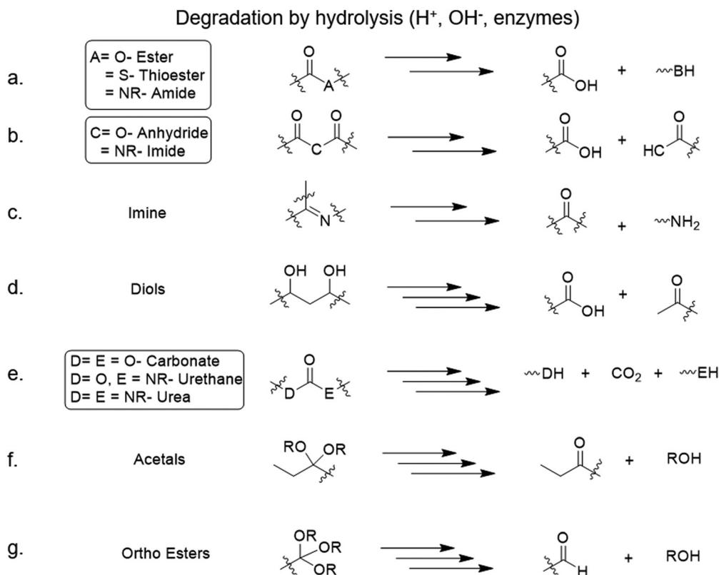
Fig. 3 Degradation mechanisms of various moieties by hydrolysis (H<sup>+</sup>, OH<sup>-</sup>, enzymes).<sup>12,23,24</sup>
