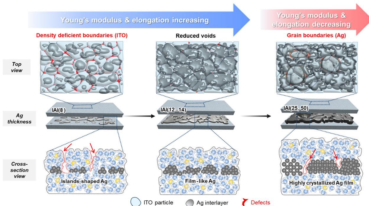
Fig. 5 Schematic of the structural changes in the IAI thin films as a function of Ag interlayer formation. The effect of the Ag interlayer and the associated mechanical properties of the IAI thin films is proposed.
