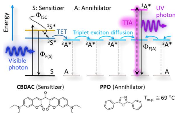
**Scheme 1** Schematic energy diagram of TTA-UC in this study. X,  $^1X^*$ , and  $^3X^*$  (X = S: sensitizer or A: annihilator) denote the ground state, excited singlet state, and excited triplet state, respectively. TET: triplet energy transfer; TTA: triplet–triplet annihilation. Bottom shows the sensitizer and annihilator selected in this study.
