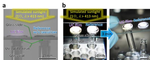
Fig. 4 (a) Schematic and (b) results of the demonstration of a utility of the UV-UC film applied to a solidification of UV curing resin with visible light ( $\lambda > 413$  nm) of 1  $\odot$  intensity at the sample position. Samples used here did not have a reflection aluminum layer on the bottom side.
