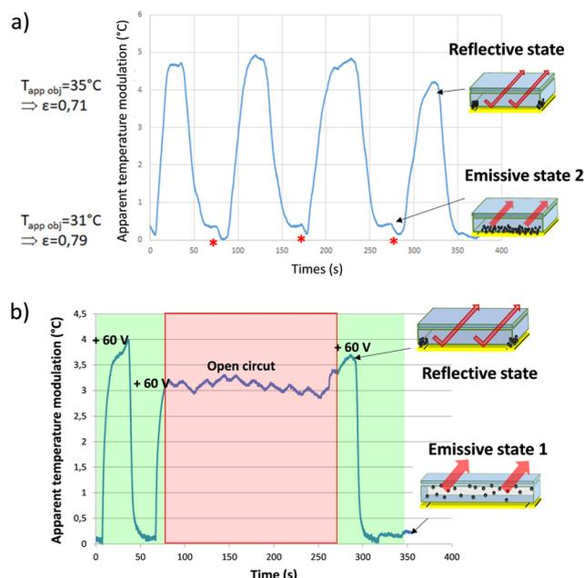
Fig. 6 (a) Performance of optimized electrophoretic cell (potential  $\pm 30 \text{ V}$  and  $F = 25 \text{ mHz}$ ). (b) Evaluation of the bistability of the electrophoretic cell (potential  $+60 \text{ V}/0 \text{ V}$  at  $F = 25 \text{ mHz}$  + open circuit). Apparent temperature observed with an FLIR camera in LWIR. The blackbody is set at  $65 \text{ }^\circ\text{C}$ .
