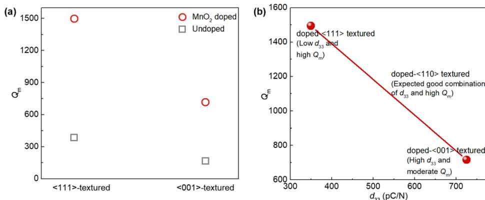
Fig. 9 (a)  $Q_m$  values of undoped and doped  $\langle 001 \rangle$  and  $\langle 111 \rangle$  textured ceramics. (b)  $Q_m$  vs.  $d_{33}$  for doped  $\langle 001 \rangle$  and  $\langle 111 \rangle$  textured ceramics.
