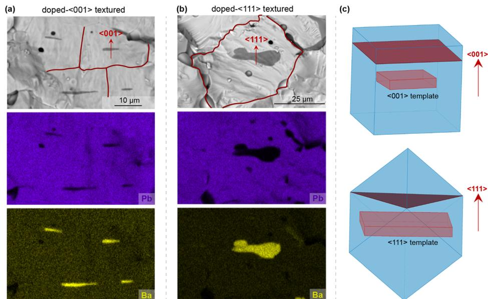
Fig. 2 (a) and (b) Cross-sectional SEM images and the corresponding EDS element mapping of doped- $\langle 001 \rangle$  and  $\langle 111 \rangle$  textured ceramics. (c) Schematic diagrams of  $\langle 001 \rangle$  and  $\langle 111 \rangle$  oriented grain growth of PIN–PMN–PT matrix on  $\langle 001 \rangle$  and  $\langle 111 \rangle$  BT templates.
