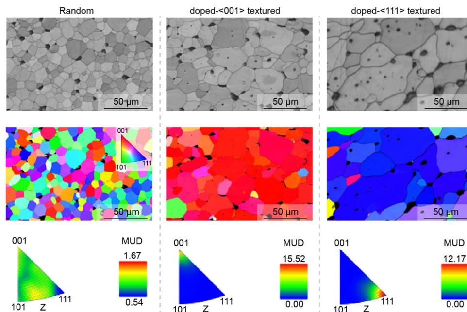
Fig. 3 SEM images of polished surface and the corresponding EBSD images of random, doped- $\langle 001 \rangle$  and  $\langle 111 \rangle$  textured ceramics. In EBSD, MUD (multiple of uniform density) is a parameter used for the statistical description of the intensity of texture. MUD value of 1 indicates randomly oriented grains and MUD value significantly  $> 1$  indicates textured grains.
