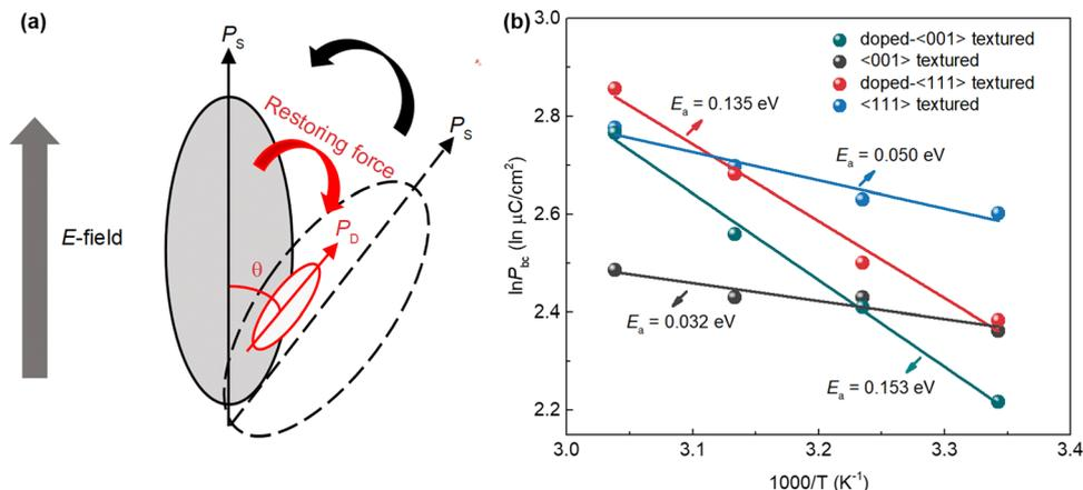
Fig. 8 (a) Schematic diagram of restricted polarization rotation induced by defect polarization  $P_D$  in acceptor-doped piezoelectric materials. (b) Plot of  $\ln(P_{bc})$  versus inverse temperature for  $\langle 001 \rangle$  and  $\langle 111 \rangle$  textured and doped  $\langle 001 \rangle$  and  $\langle 111 \rangle$  textured ceramics.
