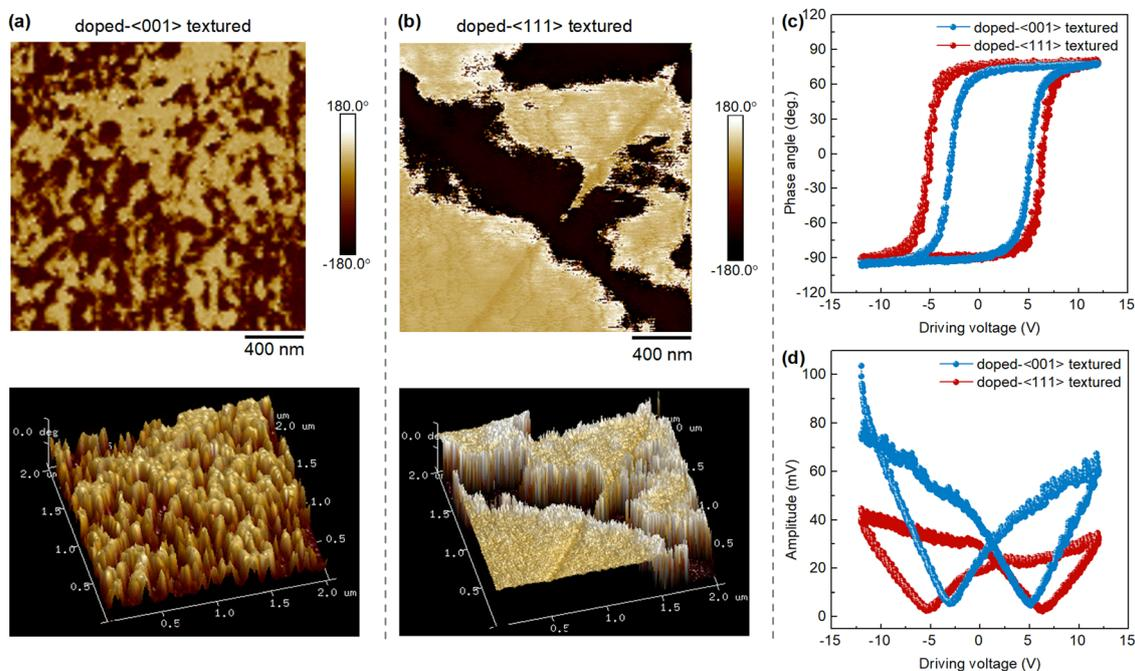
Fig. 6 (a) and (b) 2D and 3D PFM phase images of domain structure for doped- $\langle 001 \rangle$  and  $\langle 111 \rangle$  textured ceramics. (c) Microscopic piezoelectric hysteresis loops and (d) butterfly-shaped amplitude versus driving voltage curves for doped- $\langle 001 \rangle$  and  $\langle 111 \rangle$  textured ceramics.
