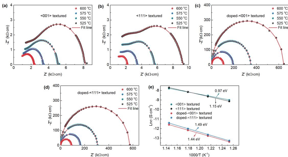
Fig. 7 (a)–(d) Temperature dependent complex impedance spectra and (e) corresponding Arrhenius plots of ionic conductivities for  $\langle 001 \rangle$  and  $\langle 111 \rangle$  textured, and doped  $\langle 001 \rangle$  and  $\langle 111 \rangle$  textured ceramics.
