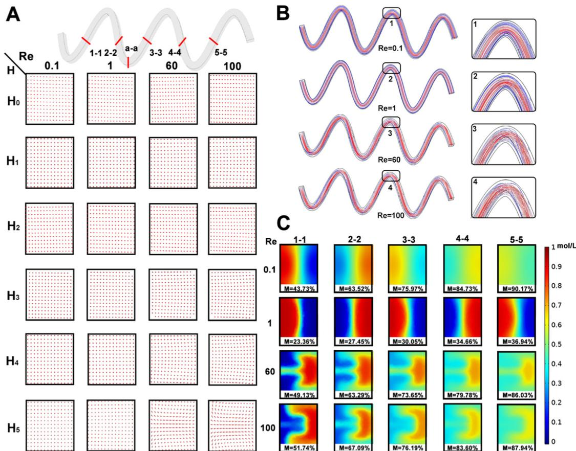
Fig. 4 (A) Flow direction of six hyperbolic curves of the micromixer at different Re for the cross-sections. (B) Streamlining of the hyperbolic micromixer's curve  $H_5$  micromixer at different Re and amplified view at channel and curves. (C) Concentration distribution of the cross-section of the hyperbolic curve  $H_5$  of the micromixer at different Re.
