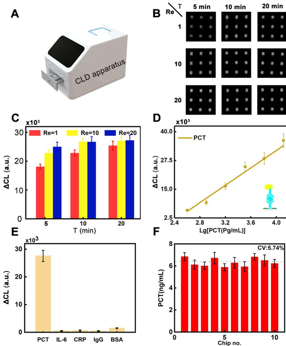
Fig. 6 (A) Chemiluminescence detection apparatus, PCT concentration of  $3.2 \text{ ng mL}^{-1}$  at different Re and incubation times for dot signal (B) and corresponding  $\Delta\text{CL}$  intensity (C). (D) Standard curve between the PCT concentration and  $\Delta\text{CL}$  intensity ( $N = 3$ ). (E) The selectivity assay of the developed for detection of PCT. (F) The stability research of the chips (No. 10) for PCT ( $6.4 \text{ ng mL}^{-1}$ ) analysis.
