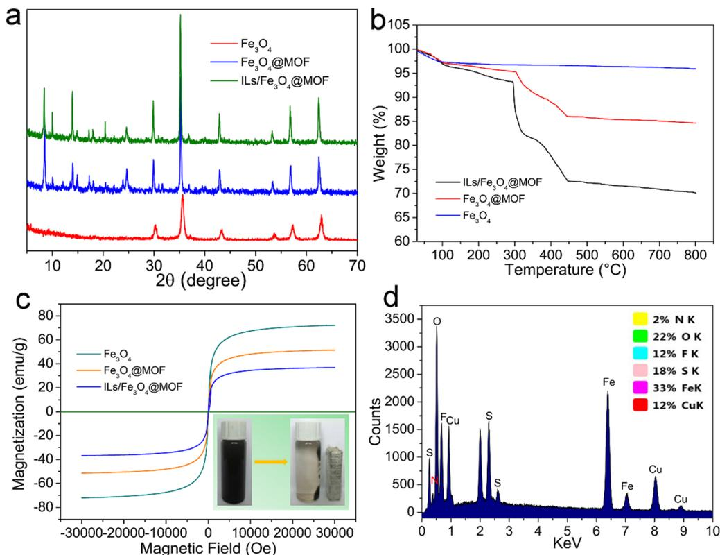
**Fig. 2** (a) XRD patterns of  $\text{Fe}_3\text{O}_4$  (red),  $\text{Fe}_3\text{O}_4@MOF$  (blue) and  $ILs/Fe_3O_4@MOF$  (green), (b) TG curves of  $\text{Fe}_3\text{O}_4$  (blue),  $\text{Fe}_3\text{O}_4@MOF$  (red) and  $ILs/Fe_3O_4@MOF$  (black), (c) magnetic properties of  $\text{Fe}_3\text{O}_4$  (blue-green),  $\text{Fe}_3\text{O}_4@MOF$  (orange) and  $ILs/Fe_3O_4@MOF$  (blue), and (d) EDS spectrum and atomic ratio of  $ILs/Fe_3O_4@MOF$ .
