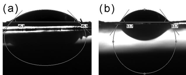
Fig. 4 Water contact angle of (a) Fe<sub>3</sub>O<sub>4</sub>@MOF and (b) ILs/Fe<sub>3</sub>O<sub>4</sub>@MOF.
