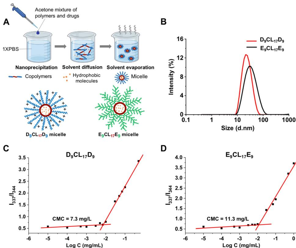
Fig. 4 Preparation and characterization of micelles. (A) Micelles were prepared via nanoprecipitation;  $D_9CL_{17}D_9$  was taken as an example. (B) The size distribution of empty micelles in an aqueous solution. (C) CMC value of  $D_9CL_{17}D_9$  (emission wavelength = 390 nm). (D) CMC value of  $E_9CL_{17}E_9$  (emission wavelength = 390 nm).
