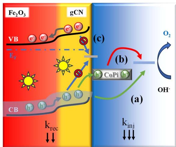
Fig. 9 Simplified model of the elementary processes taking place on the  $\text{Fe}_2\text{O}_3$ -gCN photoanode in the presence of CoPi. Photoexcited carriers move towards the semiconductor/electrolyte interface with direct water oxidation by VB holes (a), and charge transfer via a CoPi co-catalyst (b). Surface state-mediated recombination is appreciably depressed (c).
