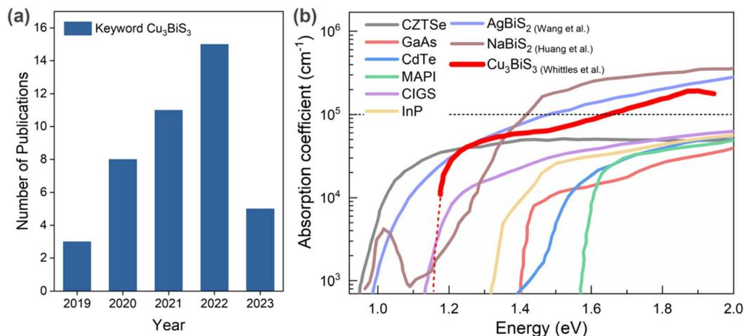
Fig. 1 (a) Number of publications on  $\text{Cu}_3\text{BiS}_3$ -related papers in the period 2019 to 2023 (source: Scopus; keyword:  $\text{Cu}_3\text{BiS}_3$ , assessed on 02 June 2023). (b) Optical absorption coefficient of Bi-based chalcogenide materials. References inserted from Wang *et al.*,<sup>13</sup> Huang *et al.*,<sup>14</sup> and Whittles *et al.*<sup>15</sup>
