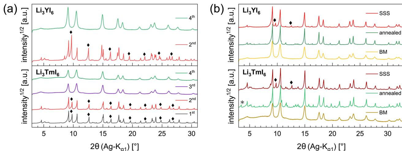
Fig. 1 Comparison of the PXRD data of  $\text{Li}_3\text{YI}_6$  and  $\text{Li}_3\text{TmI}_6$  synthesized via different routes: (a) diffraction patterns collected after every step of ball-milling. A comparison of the diffraction patterns of the different synthetic approaches (MCBM with and without subsequent annealing and SSS) is given in (b). Diamonds highlight reflections attributed to unreacted  $\text{MI}_3$  and asterisks denote the side phase MOI.
