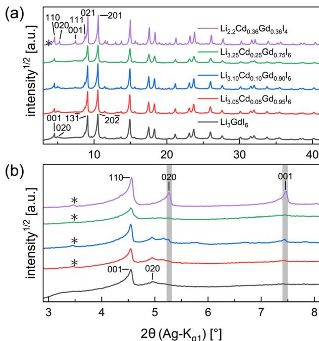
Fig. 6 Comparison of the PXRD patterns obtained for the cadmium substituted  $\text{Li}_3\text{GdI}_6$ : (a) full patterns and (b) low angle regions with selected reflection indices. The positions of the  $\text{Li}_{1.5+5x}\text{Cd}_{0.5-x}\text{Gd}_{0.5-x}\text{I}_4$ -related 020 and 001 reflections are highlighted with grey lines. The asterisks denote impurities of GdOI.
