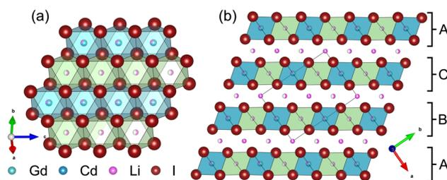
Fig. 7 (a) Mixed chain-like layer and (b) staggered stacking of the mixed chain-like and solely lithium containing honeycomb layers in  $\text{Li}_{1.5+5x}\text{Cd}_{0.5-x}\text{Gd}_{0.5-x}\text{I}_4$  with  $x = 0.14$ . While the green octahedra are exclusively occupied with lithium, the blue octahedra in the mixed chain-like layers are occupied with lithium, gadolinium and cadmium.
