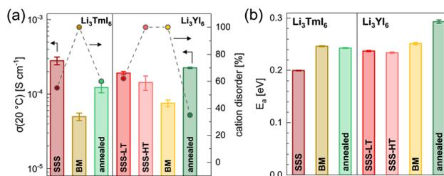
Fig. 3 Comparison of the ionic transport properties obtained from EIS for  $\text{Li}_3\text{TmI}_6$  and  $\text{Li}_3\text{YI}_6$  synthesized *via* SSS, MCBM without and with subsequent calcination. Ionic conductivities at  $20^\circ\text{C}$  and degree of intra-layer cation disorder in (a) and activation energy for ion diffusion are depicted in (b).
