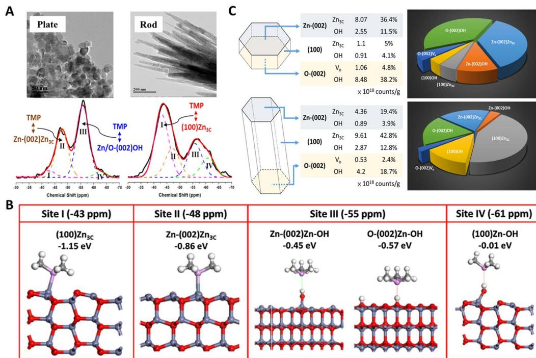
Fig. 6 (A)  $^{31}\text{P}$  NMR spectra of TMP-adsorbed plate-/rod-like ZnO crystallites. (B) DFT simulation of the adsorption configuration and energy of TMP on  $\text{Zn}_{3\text{C}}$  (I and II) and proton (III and IV) species. (C) Distribution, concentration, and percentage of various surface features on plate-/rod-like ZnO revealed by TMP- $^{31}\text{P}$  NMR.<sup>88</sup> Copyright © 2016 American Chemical Society.
