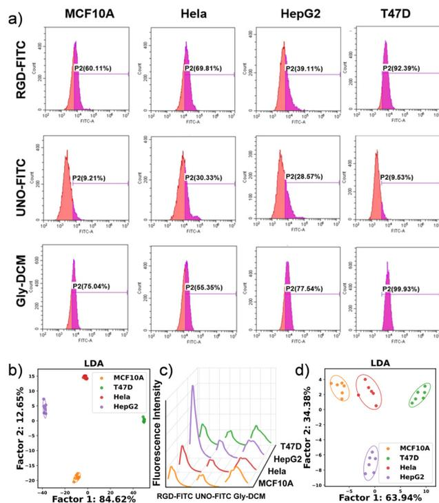
**Fig. 1** Differentiation of normal cells and cancer cells using a multi-well sensor array. (a) FCM results and (b) LDA plot of the sensor array with MCF10A, HeLa, HepG2, and T47D, respectively. (c) Fluorescence spectra and (d) LDA plot of the sensor array with MCF10A, HeLa, HepG2, and T47D, respectively.
