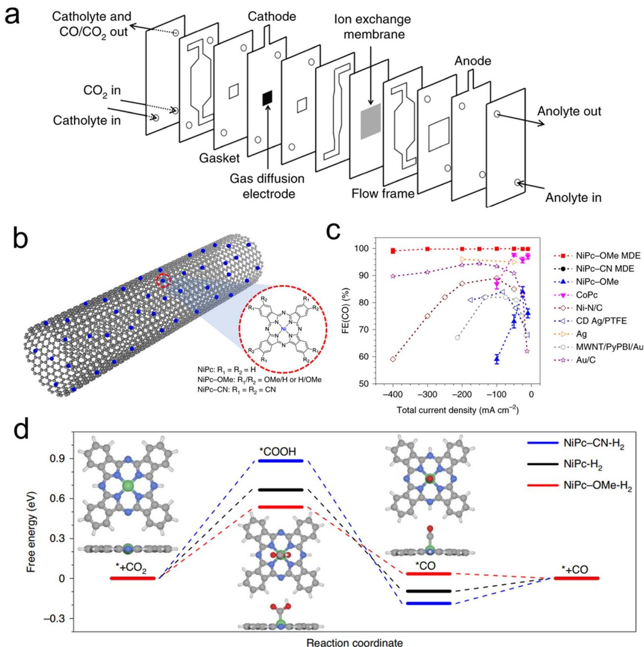
Fig. 4 The typical electrolyser configuration employing GDEs (a),<sup>61</sup> a scheme of catalyst-CNT integration (b), effects of functional groups on performance (c), and free-energy landscape of  $\text{CO}_2\text{R}$  (d),<sup>46</sup> reproduced with permission from Springer Nature copyright 2019.
