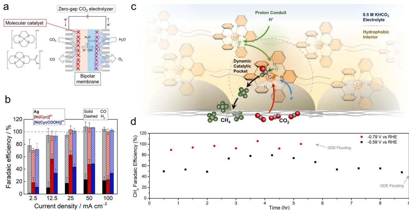
Fig. 5 Ni cyclam catalysts were integrated with bipolar membrane electrolyzers (a), in which they reduced  $\text{CO}_2$  to CO (b).<sup>74</sup> Proton shuttling enables  $\text{CO}_2\text{R}$  within a hydrophobic pocket within GDE electrodes (c) and shifts the reaction selectivity to  $\text{CH}_4$ , with a selectivity of almost unity (d).<sup>78</sup> Reproduced with permission from the American Chemical Society, copyright 2022.
