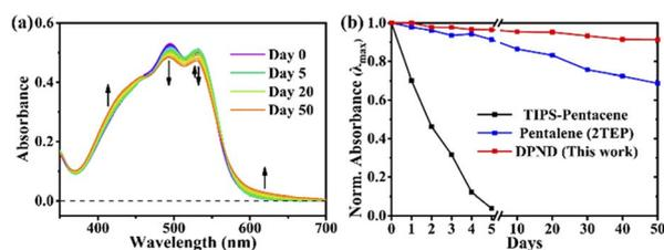
Fig. 15 Stability testing of 1h molecule: (a) steady-state absorption spectra and (b) normalized intensity of the  $\lambda_{\text{max}}$  of thin films exposed to air and light. Adapted with permission from ref. 8d. Copyright 2020 American Chemical Society.
