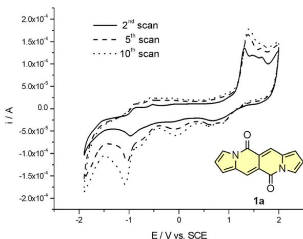
Fig. 7 Cyclic voltammogram registered for **1a** in dichloromethane in the entire range of examined potentials:  $-1800 \div 2100$  mV,  $\nu = 100$  mV s<sup>-1</sup>. Adapted with permission from ref. 18 Copyright 2016 Royal Society of Chemistry.
