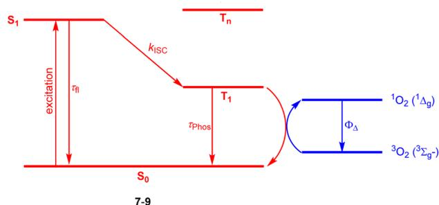
Fig. 21 Schematic illustration of energy levels and triplet sensitization in 7–9.<sup>21,60</sup>
