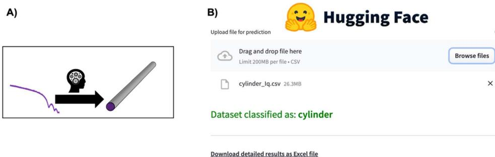
Fig. 5 (A) The SCAN<sup>74</sup> tool directly predicts structural information such as particle shape from a SAXS pattern. (B) Overview of the SCAN<sup>74</sup> tool's ease of use for predicting structural information from a SAS pattern through the Hugging Face app.<sup>75</sup> Simply click "Browse files", wait for the model to predict the structural information, and, if needed, download the detailed information in an Excel sheet.
