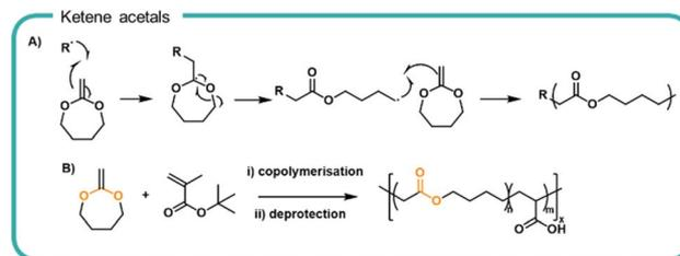
Fig. 4 (A) Schematic mechanism of the homolytic ring opening polymerisation of ketene acetal, 2-methylene-1,3-dioxepane (MDO) to form an ester-containing polymer. (B) Preparation of poly(2-methylene-1,3-dioxepane)-*co*-(acrylic acid).
