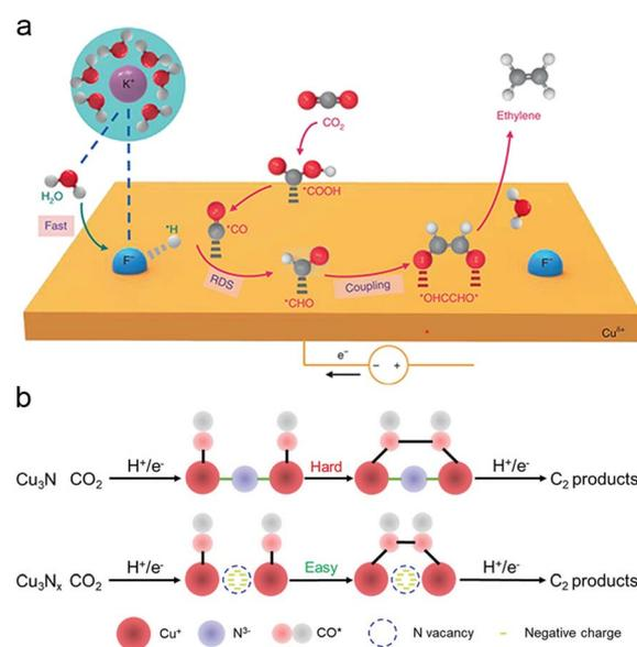
Fig. 5 (a) Schematic illustration of the possible reaction mechanism for  $C_2H_4$  generation over F–Cu catalysts. The purple, blue, red, gray, and white spheres represent K, F, O, C, and H atoms, respectively. Reproduced from ref. 93. Copyright 2020 Nature. (b) Schematic illustration of the simplified ECR mechanism towards  $C_2$  products demonstrated by the  $Cu_3N_x$  model with nitrogen vacancies. Reproduced from ref. 122. Copyright 2021 Wiley-VCH.
