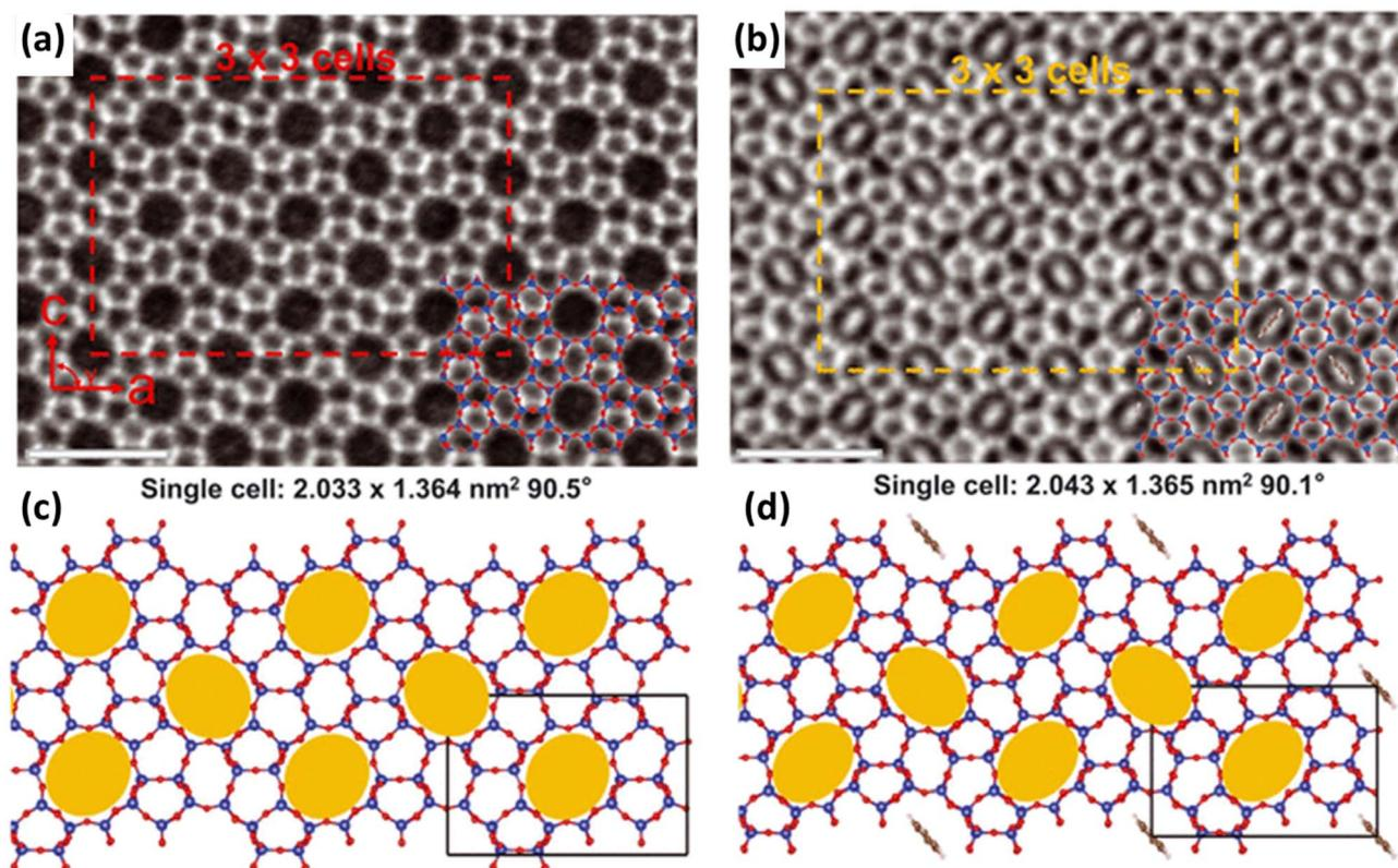
Fig. 4 Integrated differential phase contrast scanning transmission electron microscopy (iDPC-STEM) images of MFI straight channels (a) before and (b) after benzene adsorption. MFI structure flexibility is also schematically highlighted (c) before and (d) after benzene adsorption. Scale bar, 500 pm (reprinted with permission from ref. 87, copyright 2022 The American Association for the Advancement of Science).
