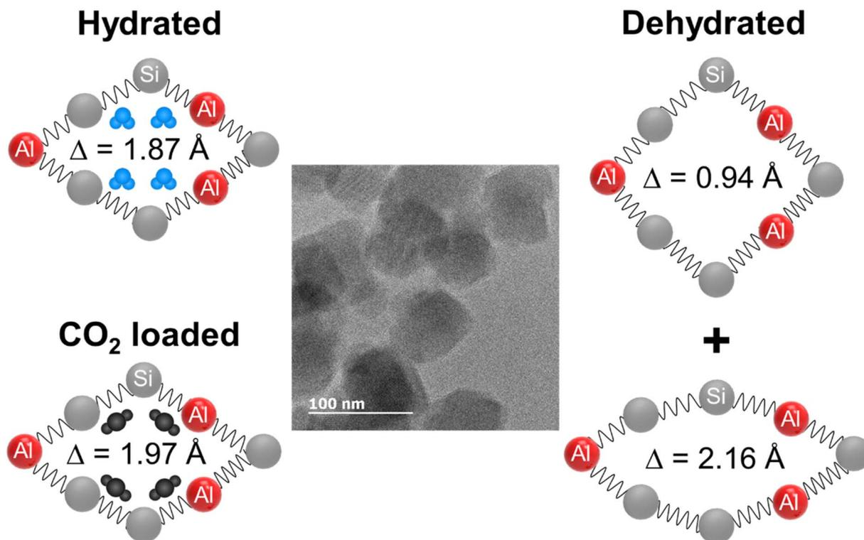
Fig. 5 Schematic illustration of reversible ellipticity of RHO nanosized zeolites upon dehydration and CO<sub>2</sub> adsorption (adopted with permission from ref. 9, copyright 2020 American Chemical Society).
