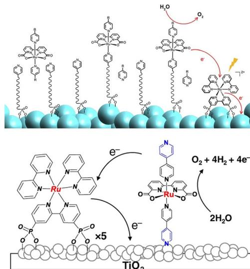
Fig. 9 Top: Coordination of a Ru(bda) WOC at  $MO_x$  surfaces exploiting a long pyridine-terminated alkyl linker; the Ru trisbipyridine photosensitizer is anchored through phosphonate linkers at the bpy. Bottom: Immobilization of a Ru(bda) WOC on  $TiO_2$  through a pyridine based anchoring group. Reprinted from ref. 92 with permission from the American Chemical Society, copyright 2018 and from ref. 93 with permission from the Nature Publishing Group, copyright 2020.
