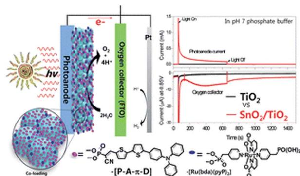
Fig. 21 Photosynthetic electrode by co-adsorbing a triarylamine photosensitizer and a  $\text{Ru}(\text{bda})$  WOC through phosphonate linkers. Reprinted from ref. 126 with permission from the Royal Society of Chemistry, copyright 2016.
