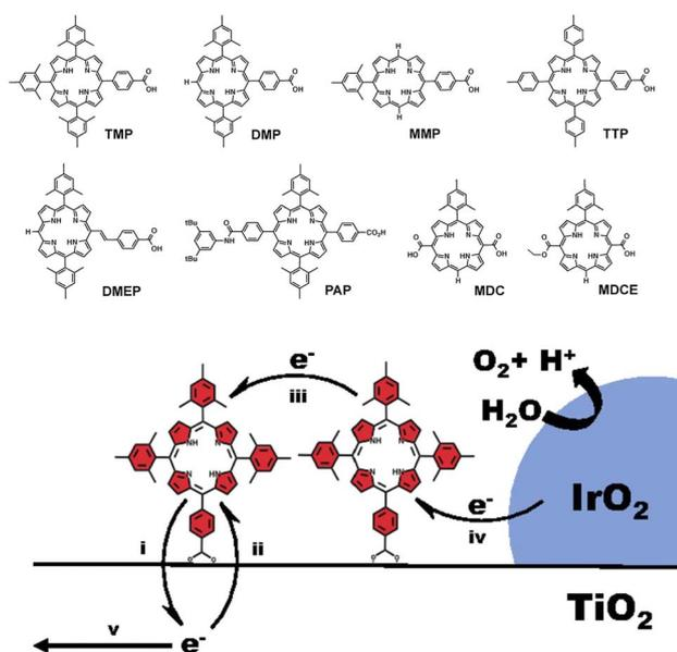
Fig. 12 Free base porphyrins considered by Mallouk and co-workers for sensitization of TiO<sub>2</sub>, in combination with an Ir oxide WOC. Reprinted from ref. 98 with permission from the *Proceedings of the National Academy of Sciences* (PNAS), copyright 2015.
