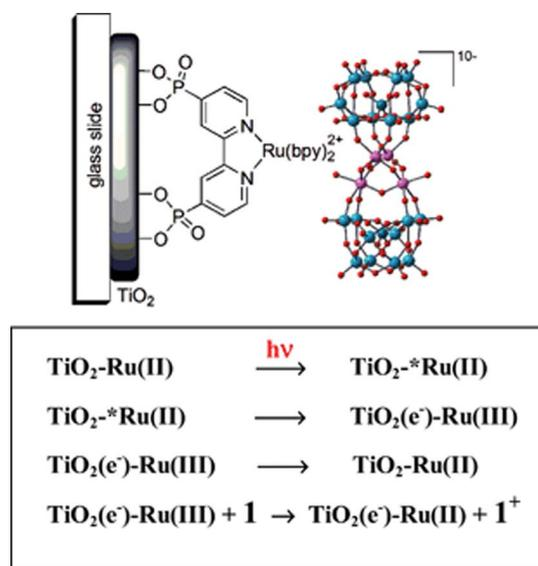
Fig. 6 Representation of a Ru trisbipyridine sensitized TiO<sub>2</sub> photoanode with a Ru<sub>4</sub>POM catalyst assembled by electrostatic interactions, and schematic view of the photoinduced electron transfer events (1 is the Ru<sub>4</sub>POM catalyst). Reprinted from ref. 79 with permission from the Royal Society of Chemistry, copyright 2010.
