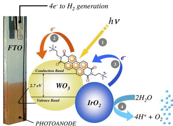
Fig. 16 A cationic perylene bisimide derivative,  $\text{PBI}^{2+}$ , absorbed on a nanostructured  $\text{WO}_3$  semiconductor and coupled to an  $\text{IrO}_x$  nanoparticle WOC, developed by Prato, Caramori and Bignozzi. Reprinted from ref. 114 with permission from the American Chemical Society, copyright 2015.
