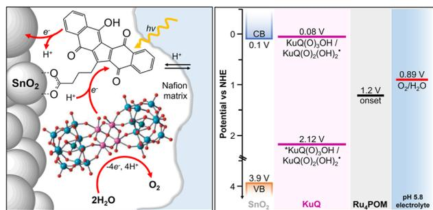
Fig. 19 Anchoring of KuQ dye onto a mesoporous SnO<sub>2</sub> surface, coupled with embedding of a Ru<sub>4</sub>POM WOC in a Nafion membrane. Energy levels of the photosynthetic assembly are shown on the right. Reprinted from ref. 123 with permission from the Royal Society of Chemistry, copyright 2020.
