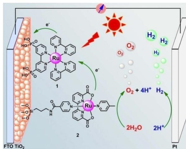
Fig. 7 Photoanode reported by Sun and co-workers, based on the ruthenium trisbipyridine dye anchored to TiO<sub>2</sub> through phosphonate linkers and a Ru<sup>II</sup>(bda) WOC functionalized with a long insulating silatrane-terminated anchoring group. Reprinted from ref. 88 with permission from the American Chemical Society, copyright 2013.
