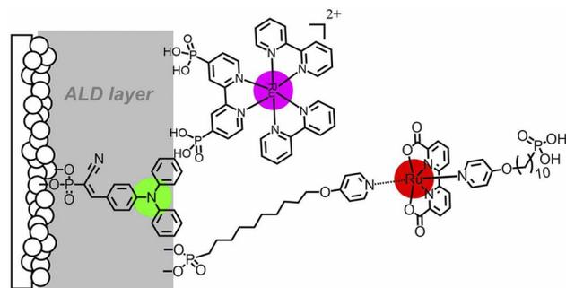
Fig. 23 Photoanodes employing a triphenylamine photosensitizer (green ball) bound to the semiconductor, a protective ALD layer used to anchor a Ru(bda) WOC (red ball) and a Ru(II) trisbipyridine redox mediator (purple ball). Reprinted from ref. 128 with permission from the *Proceedings of the National Academy of Sciences* (PNAS), copyright 2018.
