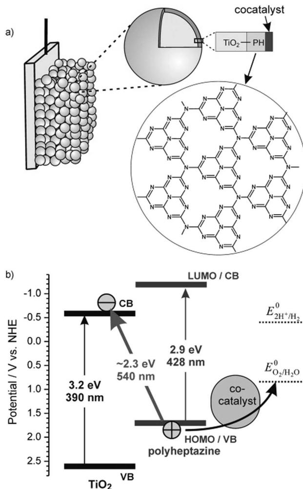
Fig. 27 (a) Hybrid photoelectrodes based on nanocrystalline  $\text{TiO}_2$  sensitized with polyheptazine and loaded with a  $\text{CoO}_x$  WOC, and (b) energy levels evidencing the direct optical charge-transfer excitation of an electron from the polyheptazine HOMO into the conduction band of  $\text{TiO}_2$ . Reprinted from ref. 134 with permission from Springer, copyright 2013.
