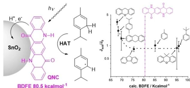
Fig. 30 Left: Schematic representation of quinacridone sensitized SnO<sub>2</sub>, capable of promoting C–H activation in organic substrates towards a Hydrogen Atom Transfer (HAT) mechanism. On the right, the photoelectrochemical response towards the organic substrate is shown, in terms of the  $J_{\text{sub}}/J_0$  parameter depending on the BDFE of the C–H bond. Reprinted from ref. 171 with permission from Wiley, copyright 2023.
