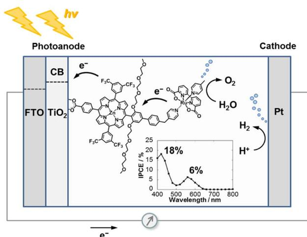
Fig. 13 A Zn-porphyrin/Ru(bda) photosensitizer/WOC dyad covalently bound to TiO<sub>2</sub>. Reprinted from ref. 104 with permission from the Royal Society of Chemistry, copyright 2016. We thank Prof. Hiroshi Imahori for providing the figure in high resolution.
