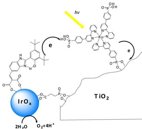
Fig. 4 Schematic representation of the photosynthetic system proposed by Mallouk and co-workers, constituted by a Ru polypyridine photosensitizer, IrO<sub>x</sub> WOC and a benzimidazole-phenol (BIP) based redox mediator, embedded onto a TiO<sub>2</sub> surface. Reprinted from ref. 72 with permission from the *Proceedings of the National Academy of Sciences* (PNAS), copyright 2012.
