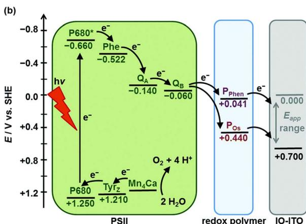
Fig. 2 (a) PSII wired *via* a redox polymer to IO-ITO electrodes (SEM image of IO-ITO is also shown), and (b) energy diagram of electron transfer events among PSII, redox polymer and IO-ITO electrode. Reprinted from ref. 62 with permission from the Royal Society of Chemistry, copyright 2016.
