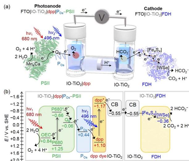
Fig. 3 (a) Representation of the photoelectrochemical cell developed by Reiser and co-workers for bias-free water oxidation and carbon dioxide reduction to formate. The photoanode is an IO-TiO<sub>2</sub>|dpp|P<sub>Os</sub>-PSII photoelectrode, while the cathode is an IO-TiO<sub>2</sub>|FDH. (b) Energy diagram. Reprinted from ref. 65 with permission from the American Chemical Society, copyright 2018.
