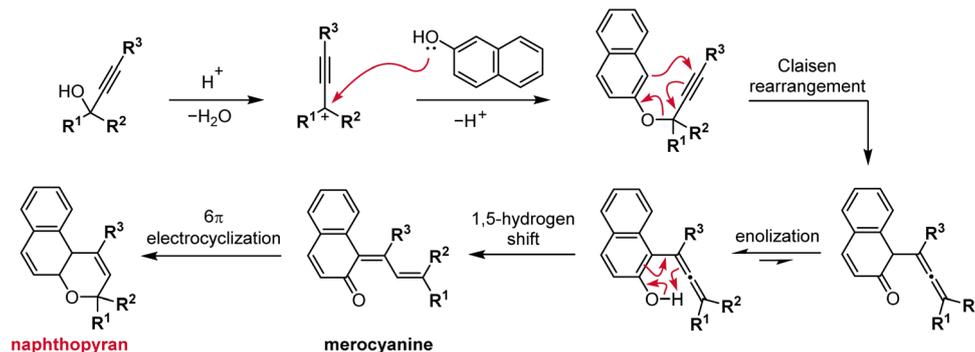
Scheme 5 Typical synthesis of naphthopyrans *via* acid-catalyzed condensation of naphthols and diaryl propargyl alcohols that proceeds through a multistep pathway. The synthesis of a 3*H*-naphtho[2,1-*b*]pyran is illustrated.
