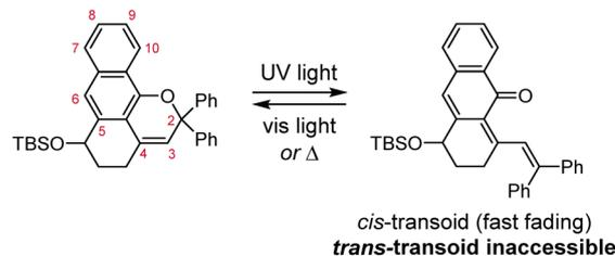
Scheme 14 Ring fusion at the 4- and 5-positions of 2*H*-naphthopyrans prevents isomerization of the *cis* merocyanine isomer to the more thermally stable *trans* configuration.<sup>220</sup>
