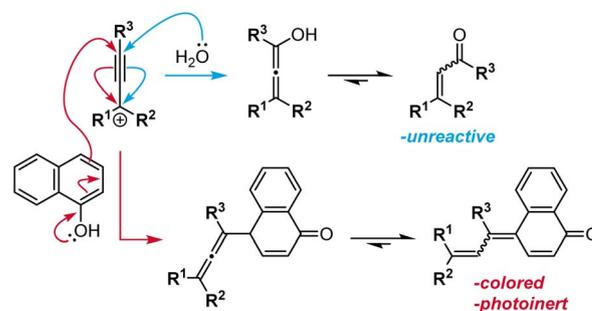
Scheme 6 Side reactions encountered in the synthesis of naphthopyrans *via* the acid-catalyzed route including the Meyer–Schuster rearrangement (top pathway, blue arrows) and conjugate addition to the propargyl cation at the 4-position of the 1-naphthol (bottom pathway, red arrows).
