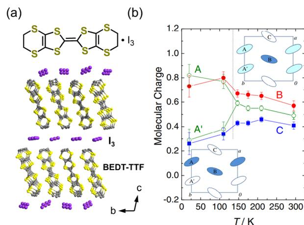
Fig. 7 (a) Crystal structure of  $\alpha$ -(BEDT-TTF)<sub>2</sub>I<sub>3</sub> (BEDT-TTF = bis(ethylene)dithio)-tetrathiafulvalene). (b) Temperature dependence of the molecular charge.<sup>43</sup> Reproduced with permission from ref. 43, The Physical Society of Japan.
