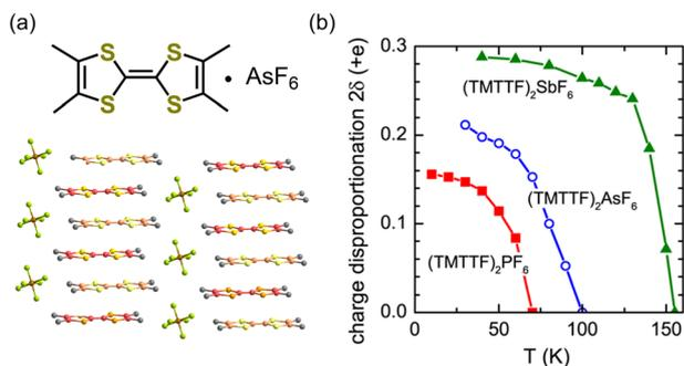
Fig. 5 (a) Crystal structure of  $(\text{TMTTF})_2\text{AsF}_6$  (TMTTF = tetramethyl-tetrathiafulvalene).<sup>21</sup> (b) Temperature dependence of the charge disproportionation ( $2\delta$ ) in  $(\text{TMTTF})_2\text{X}$ , where  $\text{X} = \text{PF}_6$ ,  $\text{AsF}_6$ , and  $\text{SbF}_6$ .<sup>34</sup> Reproduced from ref. 34.
