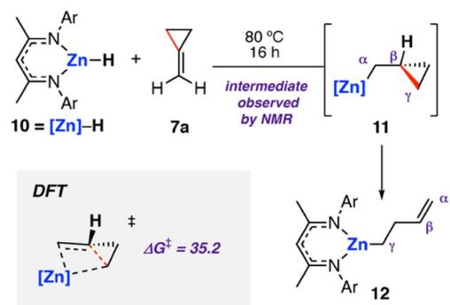
**Scheme 4** Stoichiometric reaction of zinc hydride complex **10** with methylenecyclopropane **7a**, forming the ring-opened zinc complex **12** via C–C  $\sigma$ -bond activation at Zn. Ar = 2,6-diisopropylphenyl. Energies for  $\Delta G_{298\text{ K}}^\ddagger$  in kcal mol<sup>-1</sup>.
