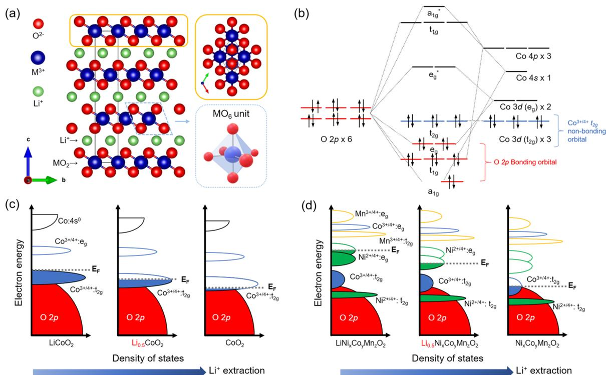
Fig. 1 Crystal and electronic structures of LTMO. (a)  $R\bar{3}m$  layered LTMO. (b) Molecular orbital hybridization of an  $\text{MO}_6$  octahedral unit in  $\text{LiCoO}_2$  (LCO). (c and d) Electronic band structures of (c) LCO and (d)  $\text{LiNi}_x\text{Co}_y\text{Mn}_z\text{O}_2$  ( $x + y + z = 1$ , NCM) by  $\text{Li}^+$  extraction.
