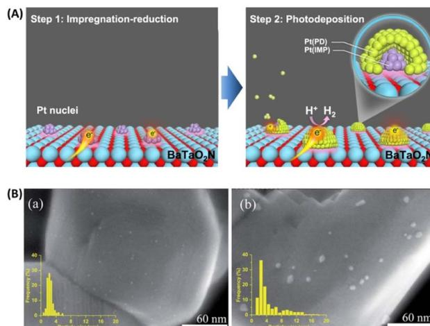
Fig. 4 (A) Schematic of sequential Pt cocatalyst deposition onto  $\text{BaTaO}_2\text{N}$ . Adapted with permission from ref. 40. Copyright 2021 Springer Nature. (B) Scanning transmission electron microscopy images and particle size distributions of (a) Na-containing and (b) Na-free Pt/ $\text{BaTaO}_2\text{N}$ . Adapted with permission from ref. 41. Copyright 2021 The Royal Society of Chemistry.
