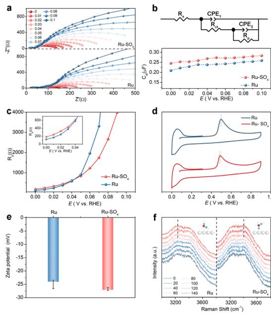
**Fig. 3** (a) Nyquist plots of Ru and Ru-SO<sub>4</sub> in the potential range from 0 V to 0.1 V. (b) The equivalent circuit and the  $C_{dl}$  at different potentials for Ru and Ru-SO<sub>4</sub>. (c) The  $R_p$  at different potentials for Ru and Ru-SO<sub>4</sub>. (d) CO stripping curves in CO-saturated 0.1 M KOH. (e) Zeta potentials of Ru and Ru-SO<sub>4</sub>. (f) *In situ* Raman spectra of interfacial water on Ru and Ru-SO<sub>4</sub> in 0.1 M KOH at 0 mV to 140 mV.
