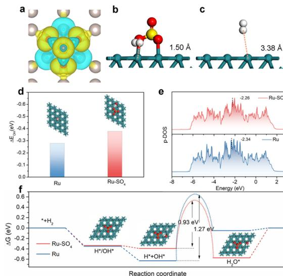
Fig. 4 (a) Calculated differential charge density for Ru-SO<sub>4</sub>. The blue and yellow areas correspond to the depletion and accumulation of electrons, respectively. The optimal theoretical structure of H<sub>2</sub> on Ru-SO<sub>4</sub> (b) and Ru (c). (d) The adsorption energy of OH\* on Ru-SO<sub>4</sub> and Ru with the corresponding optimal theoretical structure. The projected density of states (e) and the reaction pathways (f) of Ru and Ru-SO<sub>4</sub>.
