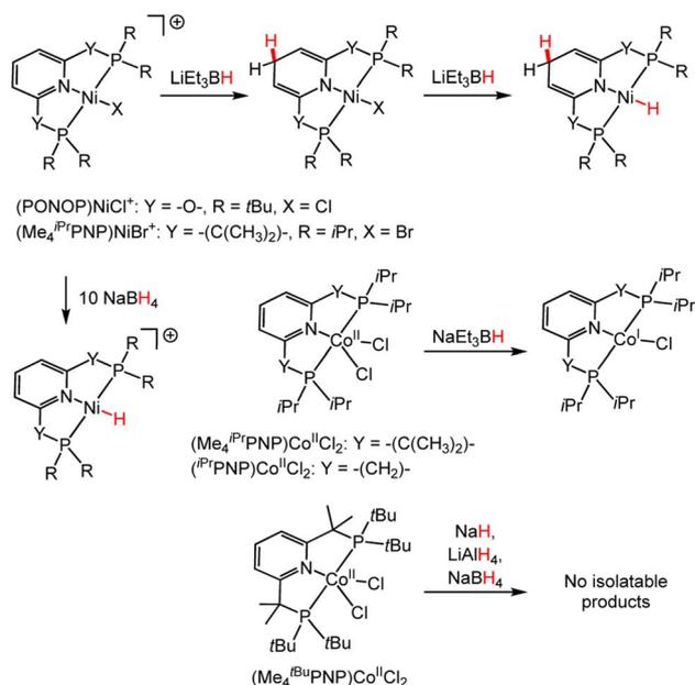
**Scheme 13** Reactions highlighting the influence of the ligands and metal ion on the HT selectivity: Ni complexes, (PONOP)NiCl<sup>+</sup>,<sup>114</sup> and (Me<sub>4</sub><sup>iPr</sup>PNP)NiBr<sup>+</sup>,<sup>87</sup> and Co complexes (Me<sub>4</sub><sup>iPr</sup>PNP)Co<sup>II</sup>Cl<sub>2</sub>,<sup>115</sup> (iPrPNP)Co<sup>II</sup>Cl<sub>2</sub> (ref. 116) and (Me<sub>4</sub><sup>tBu</sup>PNP)Co<sup>II</sup>Cl<sub>2</sub>.<sup>117</sup>
