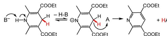
Scheme 10 (Top) The proposed mechanism for reaction of HEH with a hydride acceptor (A) in the presence of a base (B<sup>-</sup>).<sup>100</sup> For the other example in the text, the acceptor A would be BNA<sup>+</sup>; in both cases, the base B<sup>-</sup> is DBU.
