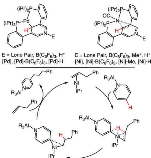
**Scheme 14** (Top): Structures of [Pd]–E and [Ni]–E.<sup>95</sup> For the CO vibrational studies to probe the electronic effects on the [Ni]–E complex, the CO was bound directly to the Ni as shown. (Bottom): Proposed mechanism for C<sub>4</sub> alkylation, which is believed to pass through a ligand-to-ligand HT rather than an oxidative insertion step.<sup>118</sup>
