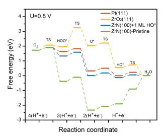
Fig. 2 Calculated free energy diagrams of the ORR at pristine ZrN(100) and ZrN(100) covered by 1 ML HO\*, Pt(111), $^{40}$  and ZrO $_2$ (111). $^{19}$  The energy barriers of the elementary steps were estimated based on the method by Dickens *et al.* $^{41}$  The potential was set to 0.8 V vs. RHE.
